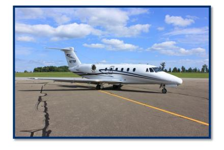
Max Range1690 nmMax Cruise Speed530 mphMax Ceiling51,000 ftMax Take-off Weight23,000 lbsMax Landing Weight20,000 lbsMin Runway Length5,000 ft
