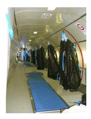
The cabin volume can be used to maximum efficiency with wall-to-wall and floor-to-ceiling loading possible. Transverse barrier nets speed up both the load and unload process and eliminate inefficiencies present with traditional throw-over net aircraft.
