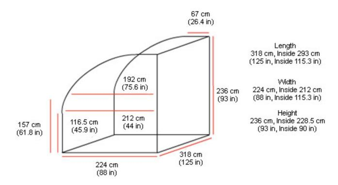
Profile for the 15 position main deck central load configuration (AeroUnion IGLU5)
