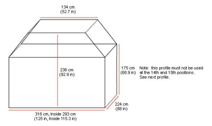
Profile type AAA (on pallet 96" x 125") at the 13th and 14th positions of the 14 position main deck central load configuration.
