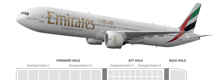
The Boeing 777-300 and 300ER is capable of carrying approximately 21,000kgs of cargo in addition to a full passenger load.
