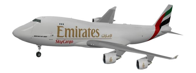
The Boeing 747-400 ERF is capable of carrying up to 117 tonnes. Its main deck-side cargo door, with a height of approximately three metres, allows the uplift of oversized shipments that cannot be accommodated in the belly-hold of passenger aircraft. The nose cargo door allows the carriage of long pieces.
